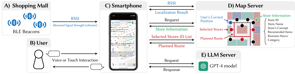
Fig. 2. The components of ChitChatGuide. A) BLE beacons are implemented at the shopping mall for localization. B) and C) Users manipulate our system installed on an iPhone 11 Pro. D) Map Server contains the information of the mall and plans a route. E) For each functionality, the system communicates with the GPT-4 model on an LLM server.
