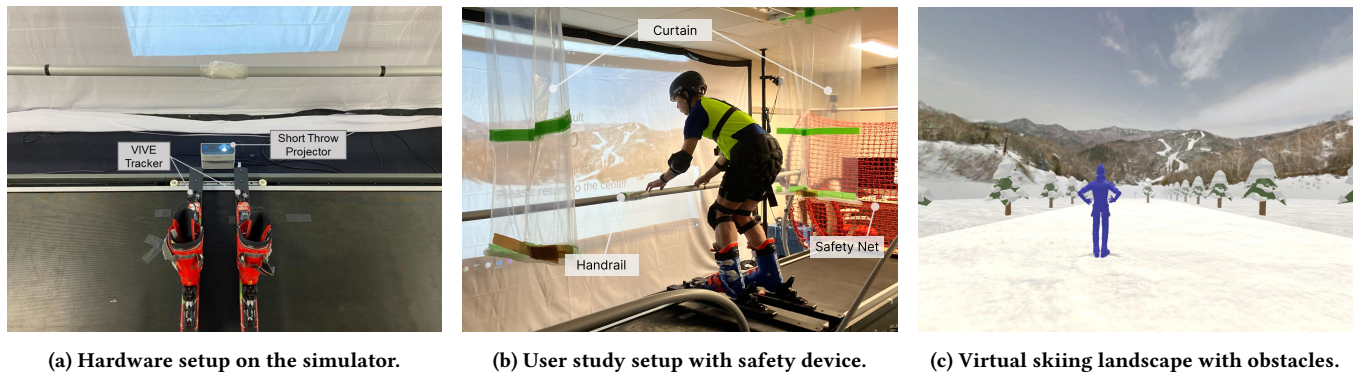
Figure 4: The setup of the system in an indoor environment.
